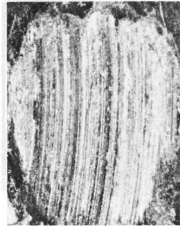
FIG. 7 Typical Test Ball Scars—After Removal
