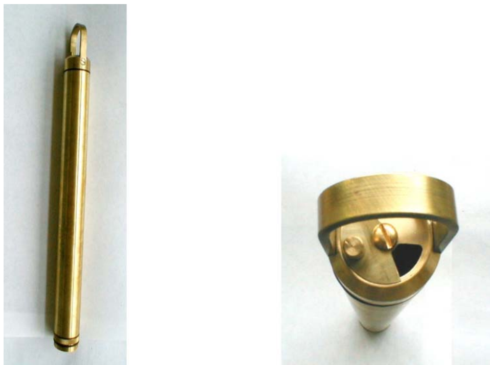
FIG. 28 Example of Closed System Restricted Flow Sampler
