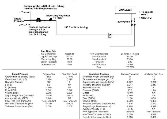
FIG. X1.2 Vaporizing Regulator Near Tap
