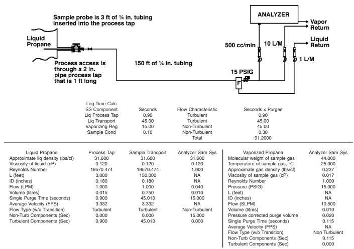
FIG. X1.3 Vaporizing Regulator Near Analyzer
