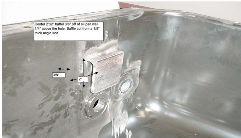
(b) Internal Modifications
