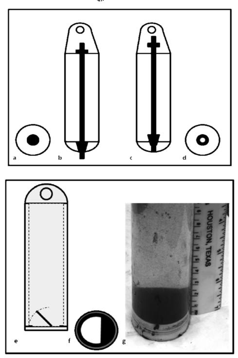
(a) closed-thief sampler; bottom-view; closed-position
