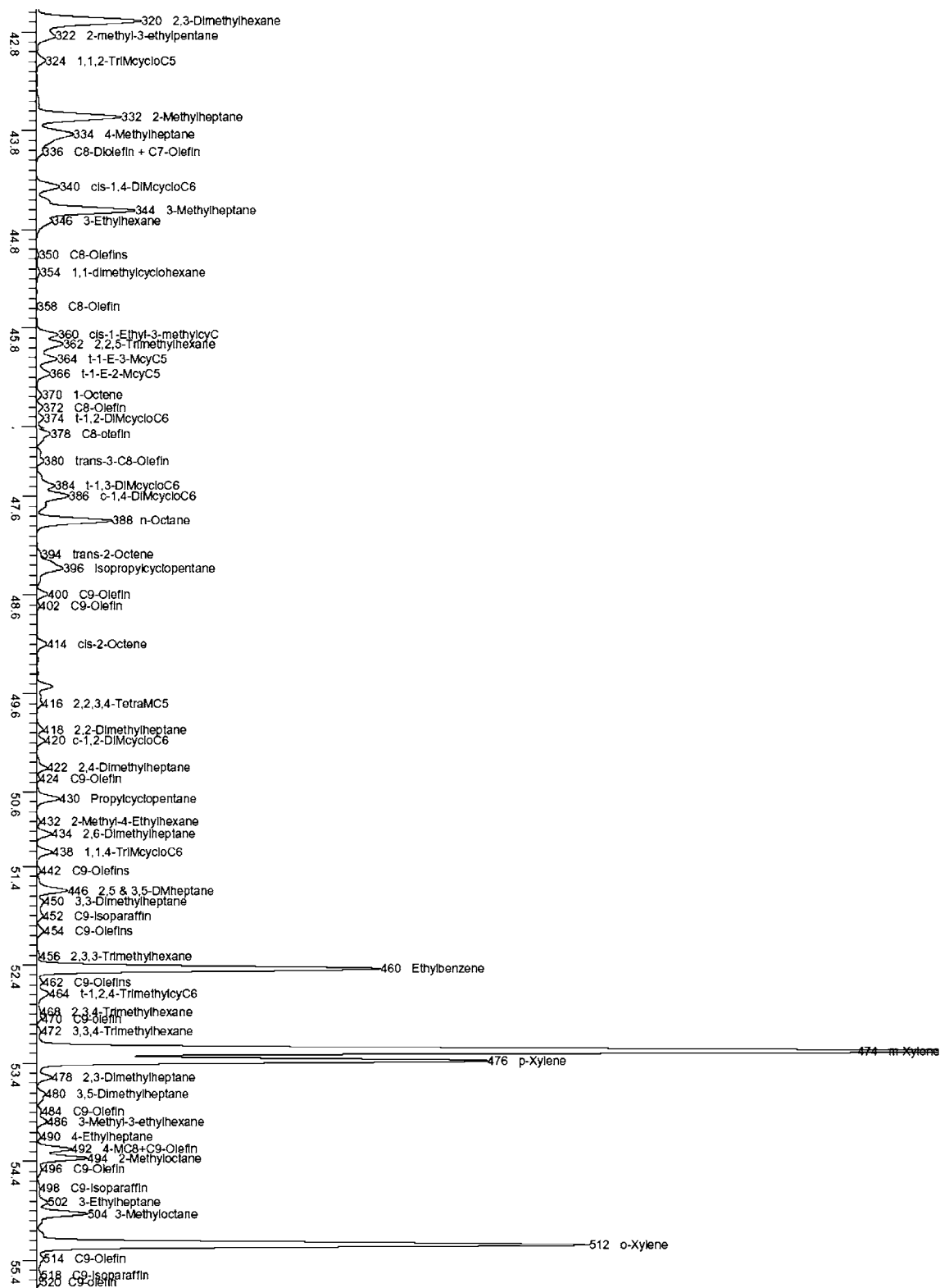
FIG. X2.9 Detailed Chromatogram for CGSB0496 Reference Gasoline (42.5 – 55.5 min)
