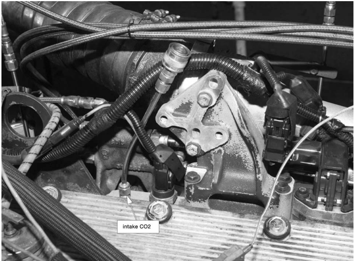
FIG. A4.14 Intake Manifold CO 2 Probe Location
