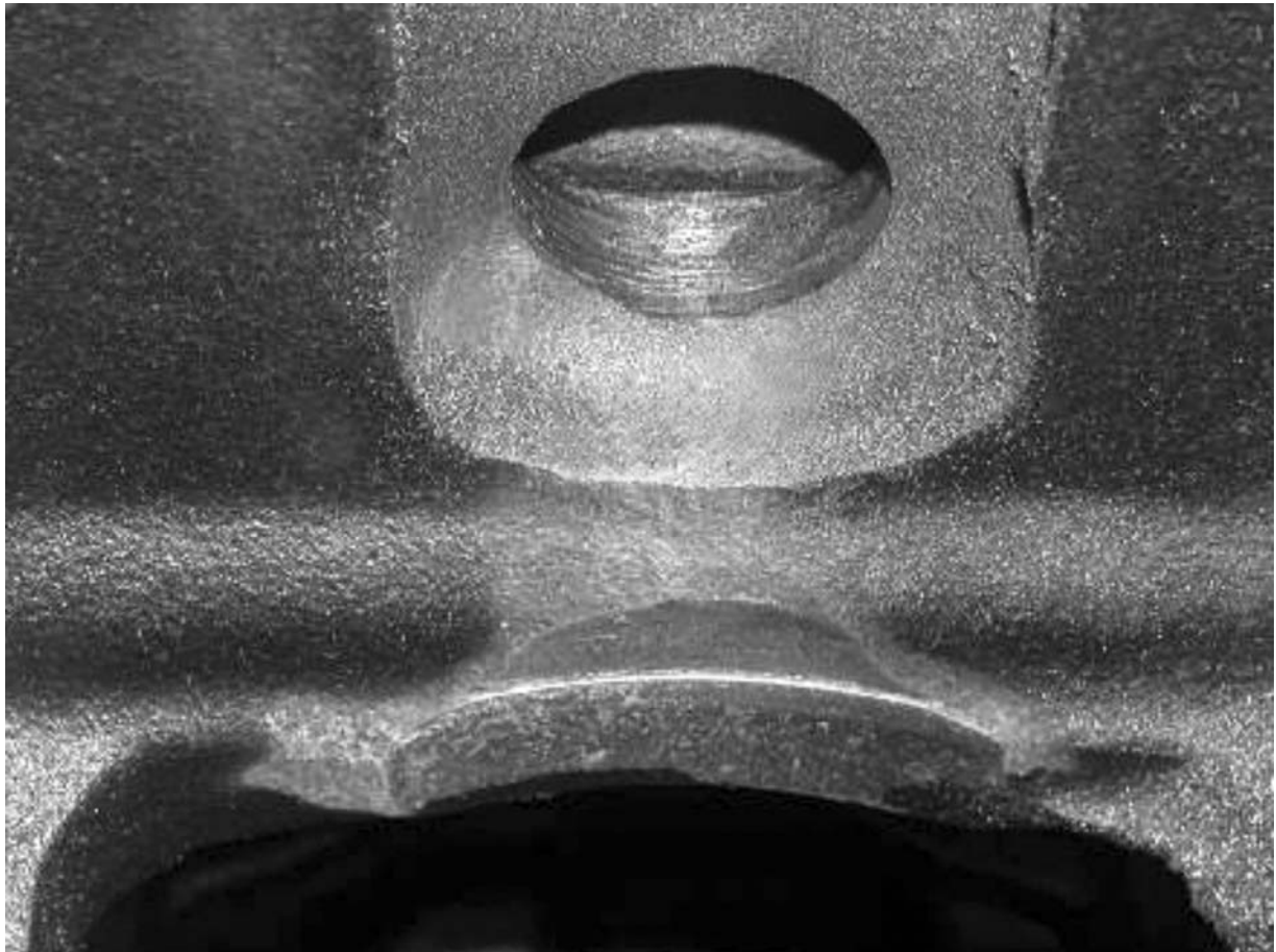
FIG. A4.17 Finished Hole in Wall of Oil Capacitor
