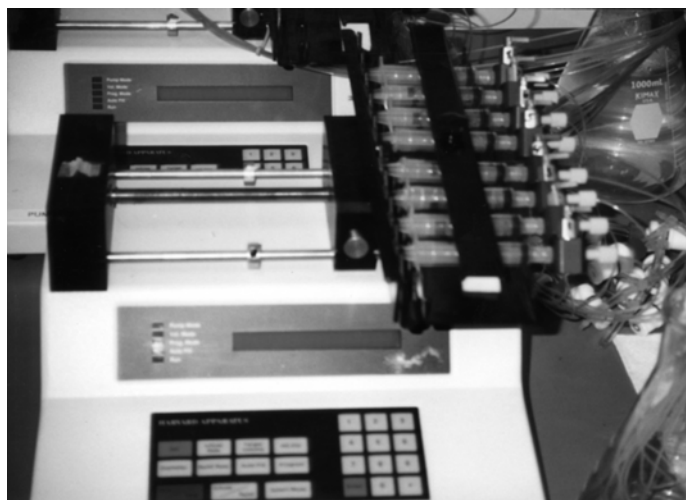
FIG. 3 Photograph of Acid Delivery System
