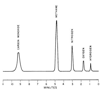
Column: 2-m by 6-mm inside diameter Type 13× molecular sieves, 14 to 30 mesh Temperature: 35°C
